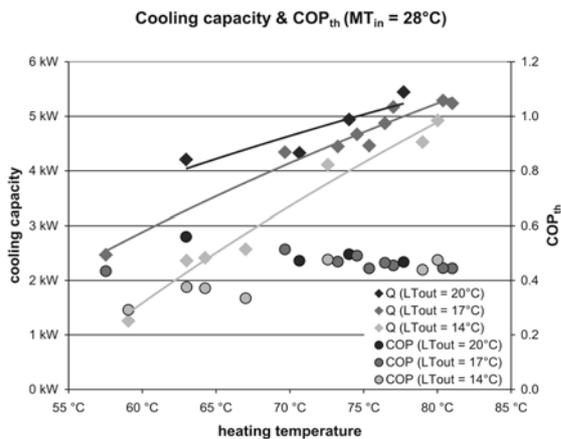
Figure 6 Measured cooling capacities and COP versus heating temperature
