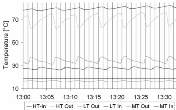
Figure 1 Periodical course of temperatures in the three external circuits passing through the heat pump
