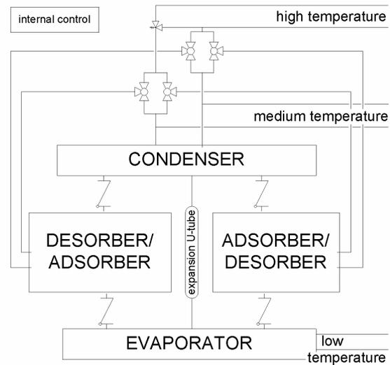
Figure 2 Schematic plan of the chillii® STC adsorption heat pump including the hydraulic switching unit
