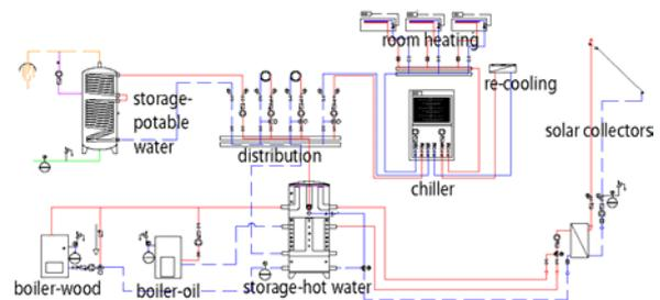
Figure 5 Simplified schematic view of the solar heating and cooling plant at CitrinSolar, Germany
