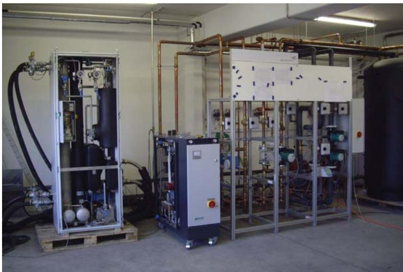
**Figure 3: Test Stand at SolarNext with the absorption chiller (Source: SolarNext)**
