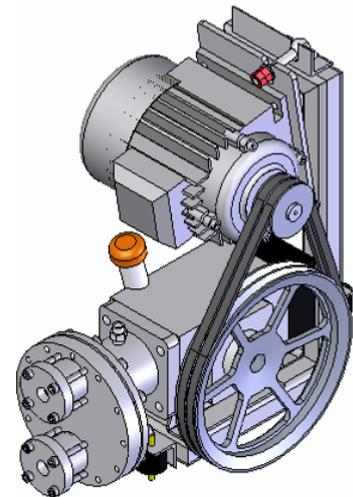
The diaphragm head with the poppet valves is put on commercially available medium pressure piston pump. The free running diaphragm is moved by oil pad. The driving power transmission takes place via two v-belts from a 0.55 KW asynchronous engine (power consumption approximately 0.25 kW). The intake pressure and the outlet pressure are 2 to 20 bar, respectively.
