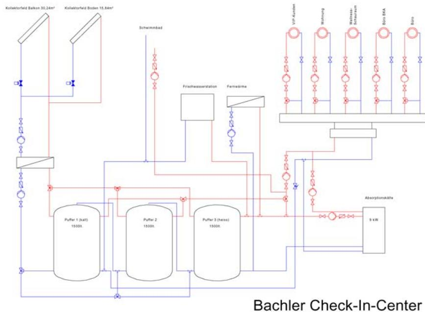
Figure 4: Simplified schematic view of the solar heating and cooling plant at Bachler Austria (source: Steiner-Haustechnik)
